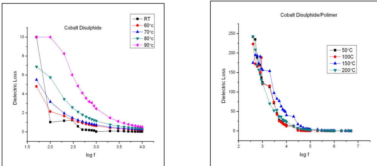
Fig. 6. log f versus Dielectric Loss for pure  $\text{CoS}_2$  and  $\text{CoS}_2$  in polymer matrix nanoparticles
