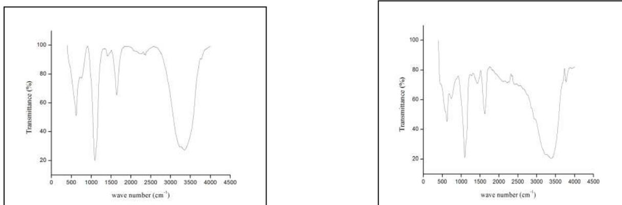
**Fig. 2. FTIR spectra of pure pure  $\text{CoS}_2$  and  $\text{CoS}_2$  in polymer matrix nanoparticles**
