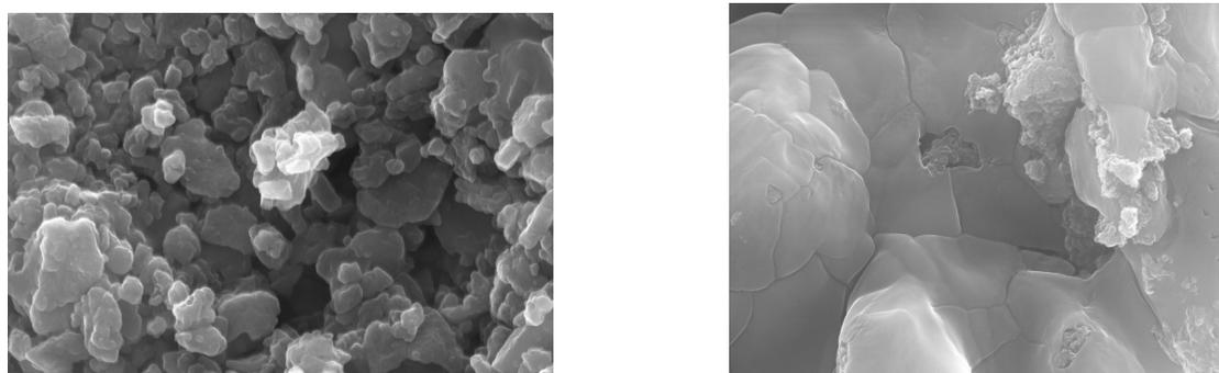
**Fig. 3. SEM image of pure  $\text{CoS}_2$  and  $\text{CoS}_2$  in polymer matrix nanoparticles**
